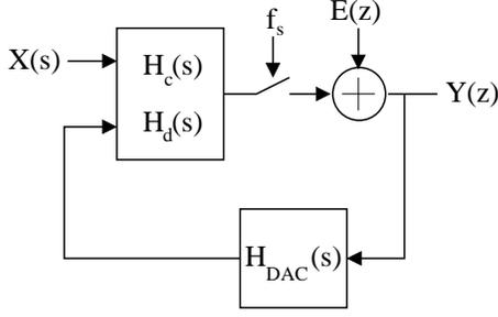
Fig. 2. A general model of a  $\Sigma\Delta$  modulator with the open-loop filter ( $H_c(s)$ ), the loop filter ( $H_d(s)$ ) and the feedback DAC filter ( $H_{DAC}(s)$ ).
