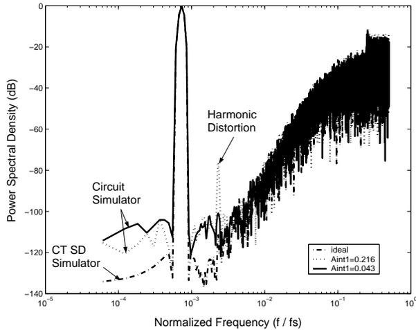
Fig. 6. Comparison between ideal system-level  $\Sigma\Delta$  simulation and circuit level simulation.
