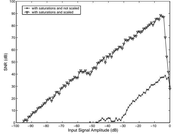
Fig. 4. 6th order CRFF, OSR=64, points=16384,  $f_{input} = \frac{13}{f_{sampling}}$
